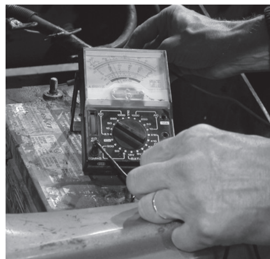
A fully-charged battery should read 12.6 v.
