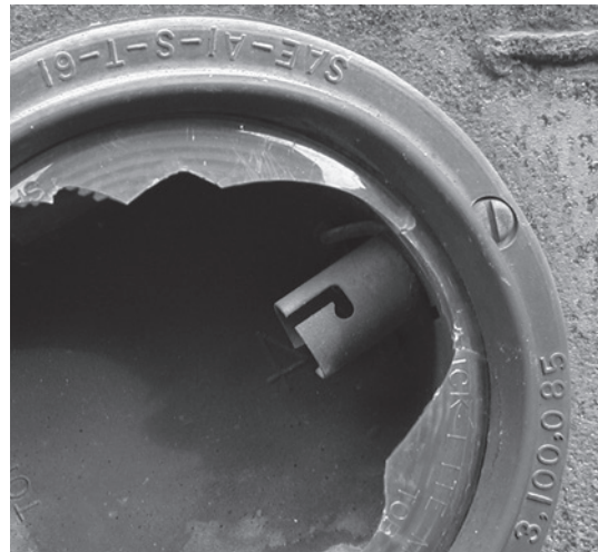
The last common cause of lamp failure is damage from road debris impact, vandalism or collision with fixed objects.
