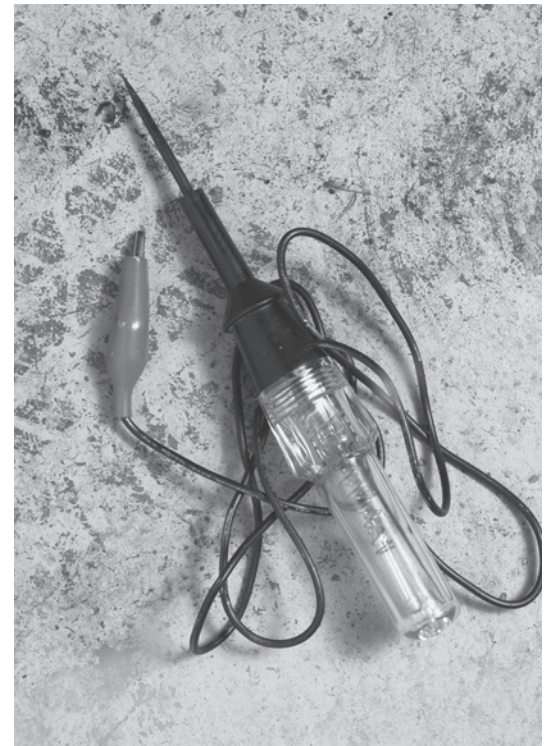
Never use the pointed tip of the tester to puncture the insulation on the wire you are testing.
