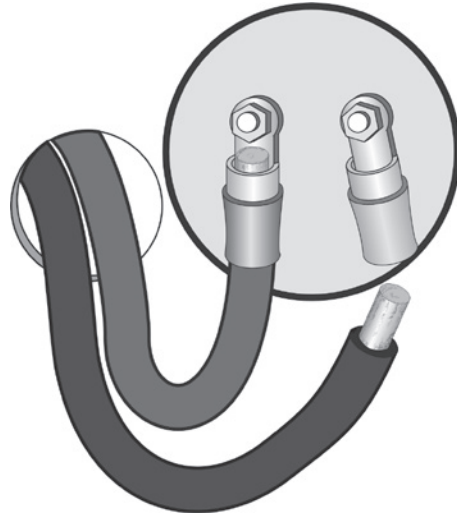
Vibration can cause connections to come apart and fail.
