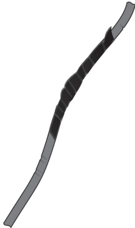
Too many splices, and splices with inadequate protection are a source of problems.
