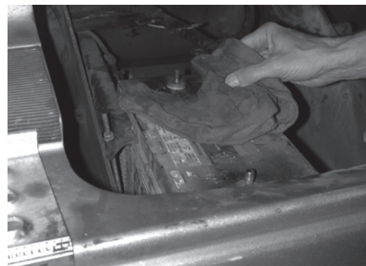
Clean up spills of electrolyte thoroughly, especially around the top and connections.
