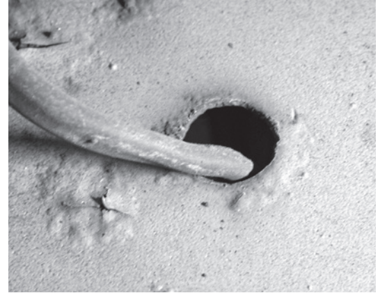
Avoid situations where wiring is in contact with sharp edges or abrasive surfaces.
