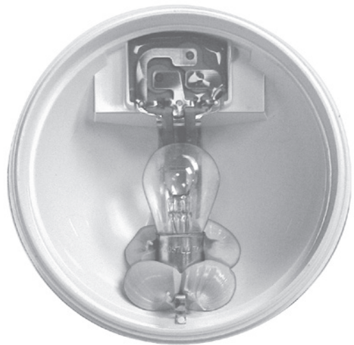
Grote Gel-Mount®, a soft cushioning material is applied around the base of the bulb to dampen vibration and shocks that could cause the bulb to fail.
