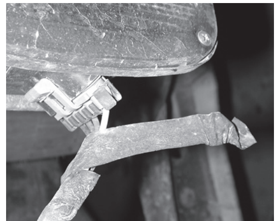
Standard electrical tape doesn't hold up well under road conditions. It has a tendency to lose its grip and come loose.
