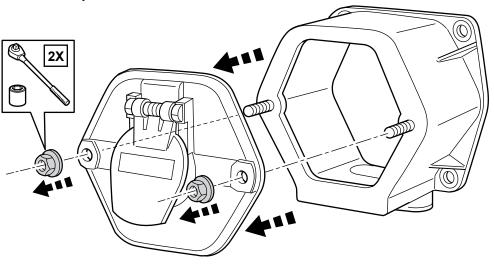
7) Remove the temporary nut holding the connector plate. Mount the Hex Box housing to the base plate and secure with four (4) nuts. Be sure to insert the rubber grommet into the opening at the back of the Hex Box housing.
