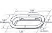
THEFT-RESISTANT MOUNTING FLANGE FOR OVAL LAMPS
