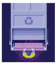
For applications which commonly have work taking place behind the vehicle, like on recycling trucks or tow trucks, we recommend two Grote WorkShield units be installed pointing inward to the center of the back of the vehicle.
