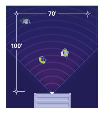
Grote WorkShield lamps create a triangular work zone that is approximately 3,000 square feet in size. It is important to ensure that the lamps are mounted so that workers (and high visibility materials) are operating in the center of this work zone. This will ensure maximum visibility.
