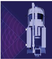
Service trucks or boom trucks may consider mounting the lamps at two locations on the vehicle so they converge at the center point and ensure maximum coverage and illumination of the work zone.
