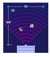
Grote HINVII lamps create a triangular work zone that is approximately 3000 square feet in size. It is important to ensure that the lamps are mounted so that workers (and high visibility materials) are operating in the center of this work zone. This will ensure maximum visibility.
