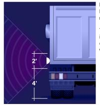
It is recommended that Grote HINVII lamps are mounted at a height range of 48" to 72" off the ground.
