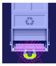
For applications which commonly have work taking place behind the vehicle, like on recycling trucks or tow trucks, we recommend two Grote HINVII units be installed pointing inward to the center of the back of the vehicle.
