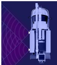
Service trucks or boom trucks may consider mounting the lamps at two locations on the vehicle so they converge at the center point and ensure maximum coverage and illumination of the work zone.
