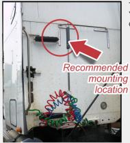
Select a mounting location vertically as high as possible to the left (driver's side) that will allow tying into a rib and without interference. There are a variety of mounting options for the EZ Claw Truck system. You may find you already have a bracket or location that will only require drilling two 3/8" holes at a 45 degree angle.
