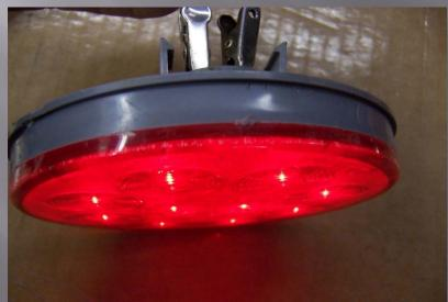
Stop Tail Turn Lamp, 01-5325-23 Test Dim And Bright Functions
