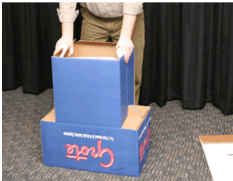
Step 7: Flip the bin over and fold down the floor tabs for added stability
